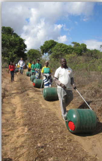
Hippo rollers, designed in Africa, allow people to collect, transport and store five times more water than a single bucket by simply rolling them along the ground. The savings in time and energy, as well as the positive social impact, are far reaching.
